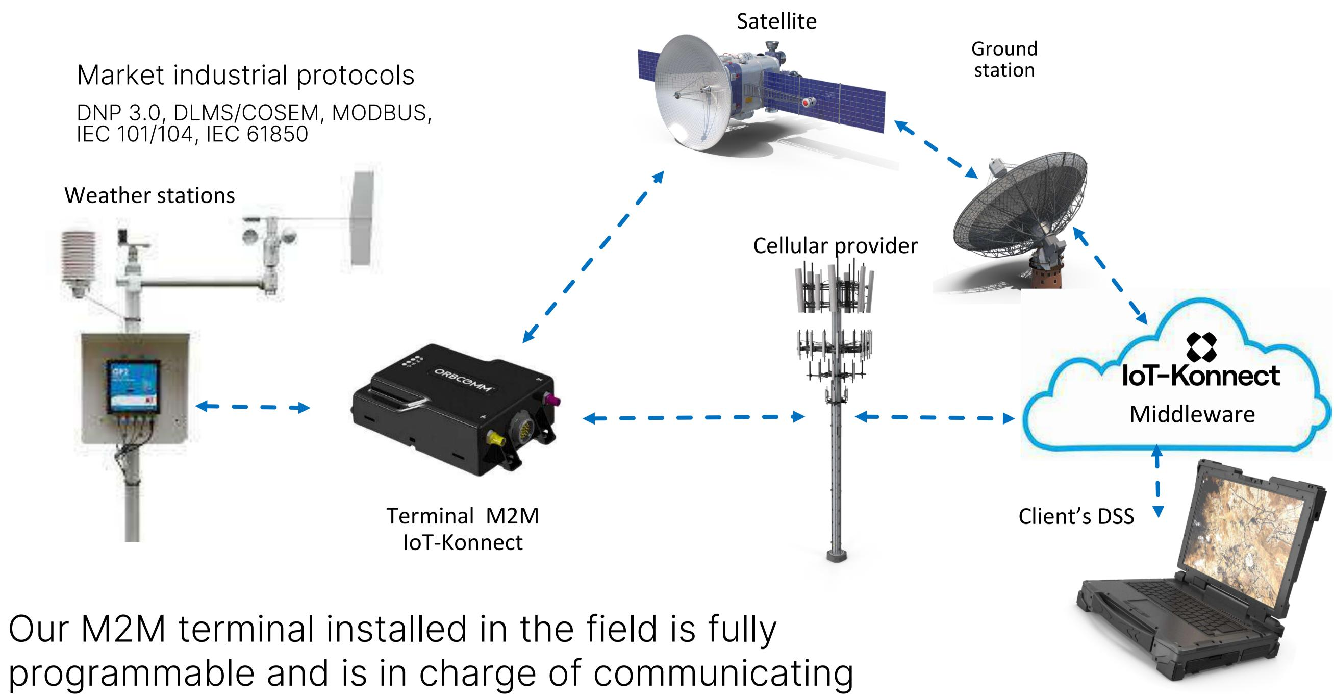
our M2M terminal installed in the field is fully programmable and is in charge of communicating the slave device with your SCADA or meteorological data analysis and processing software. The signals are sent through a variety of communications options up to our middleware and then to your DSS software, using encrypted and secure channels.
